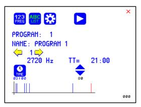
A touch on the icon opens the menu "ABC". The example chosen for this manual shows the program number, the program name and its first frequency. The timer is set for 03:00 minutes, the total time shows 21:00 minutes for a program total of 7 frequencies.
