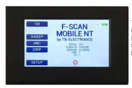
The F SCAN® MOBILE NT provides a link between the F-SCAN® COMPACT and the F-SCAN®3 NT. The device has a colored touchscreen instead of a keyboard. Settings can be changed and functions operated by touching the respective symbols on the touchscreen. Operation is easy to learn.
